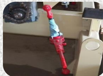
MANUAL HEIGHT ADJUSTMENT
