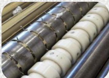
SHELL, PICKER & TRANSFER ROLLER ASSEMBLIES
