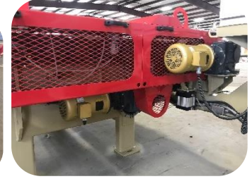
DRIVE SYSTEMS FOR FEED & TRANSFER ROLLER
